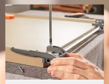
Locking unit and synchronisation shaft Attach the locking unit to the synchronisation shaft. It has to be flush with the pull-out shelf.
